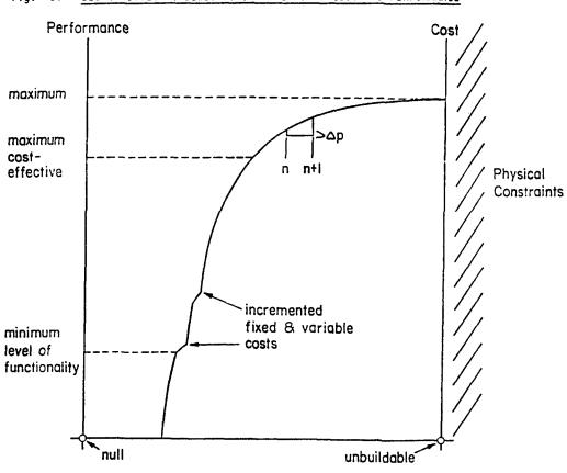
Fig. DS DESIGN STYLES (IDEOLOGIES) IN TERMS OF COST AND PERFORMANCE
