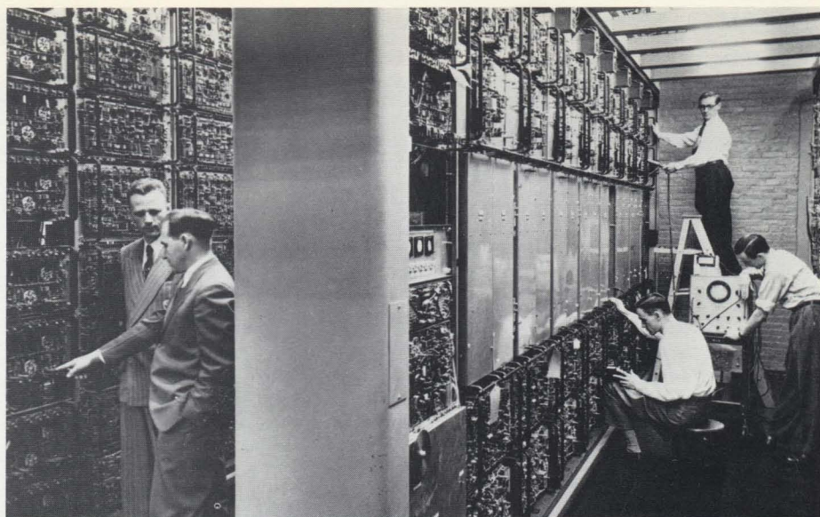
From left to right: Jay Forrester, Norman H. Taylor, John A. O'Brien, Charles L. Corderman, and Norman H. Daggert inspect the open, high voltage Arithmetic and Electrostatic Storage Racks characteristic of computer equipment in the early 1950s.
