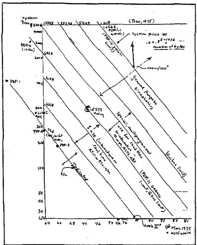
Fig. 2 System price vs. time for various memory sizes and system types (Bell, 1975).
